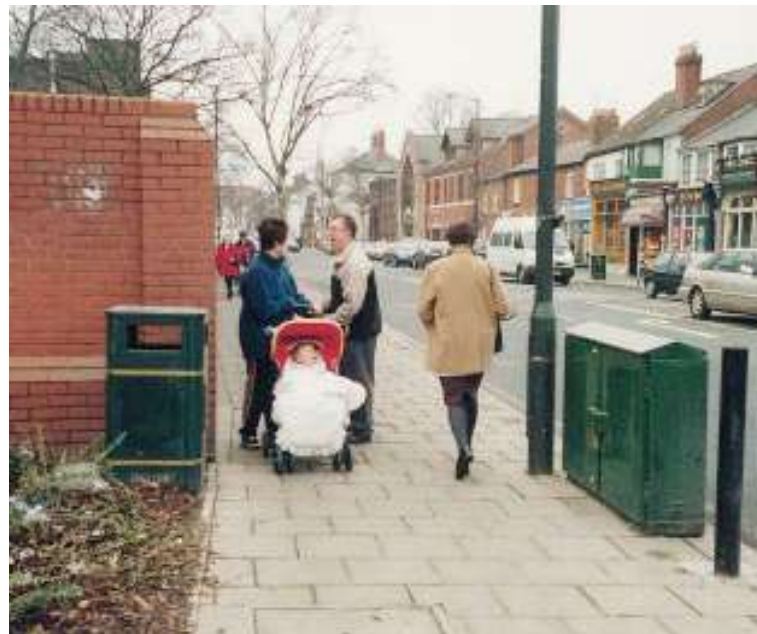
Well-positioned street furniture maximises the usable space for pedestrians. Courtesy: Ove Arup/David Davies.
